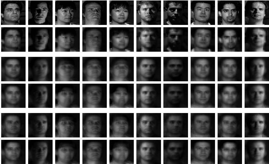
Figure 9: Pairs of rows from top to bottom: Original face images ( 60 \times 60 pixels) and sub-sampled images ( 20 \times 20 pixels); super-resolution images produced by KHA after one resp. four passes through the data set; likewise for KHA-SMD.
