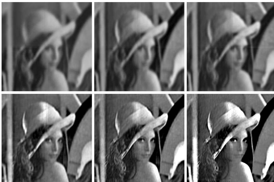
Figure 7: Reconstructed Lena image after (left to right) 1, 2, and 3 passes through the data set, for KHA with constant gain \eta_t = 0.05 (top row) vs. KHA-SMD (bottom row).
